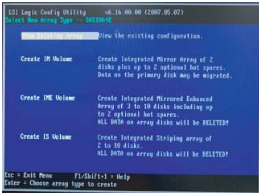
Figure 6-4 Logic MPT Setup Utility – RAID properties
