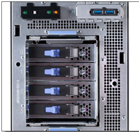
Figure 34. Simple-swap drive bays of the compact tower models (accessible with the front bezel removed)
