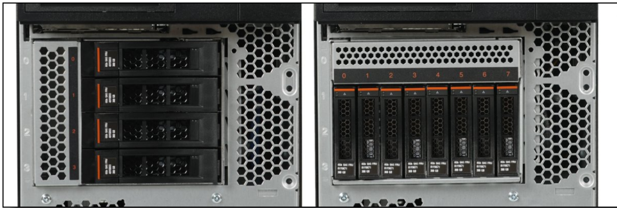
Figure 35. Hot-swap drives that are supported in standard tower models with hot-swap power supplies (front bezel removed) - 4x 3.5-inch (left) or 8x 2.5-inch (right)
